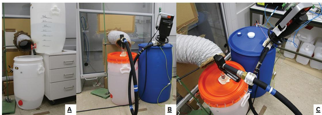
**Figure 3.** Self-assembled local exhaust ventilation system (LEV, 'Elephant trunk') using a fume hood. A: Gravity transfer; B and C: drum pump transfer.
