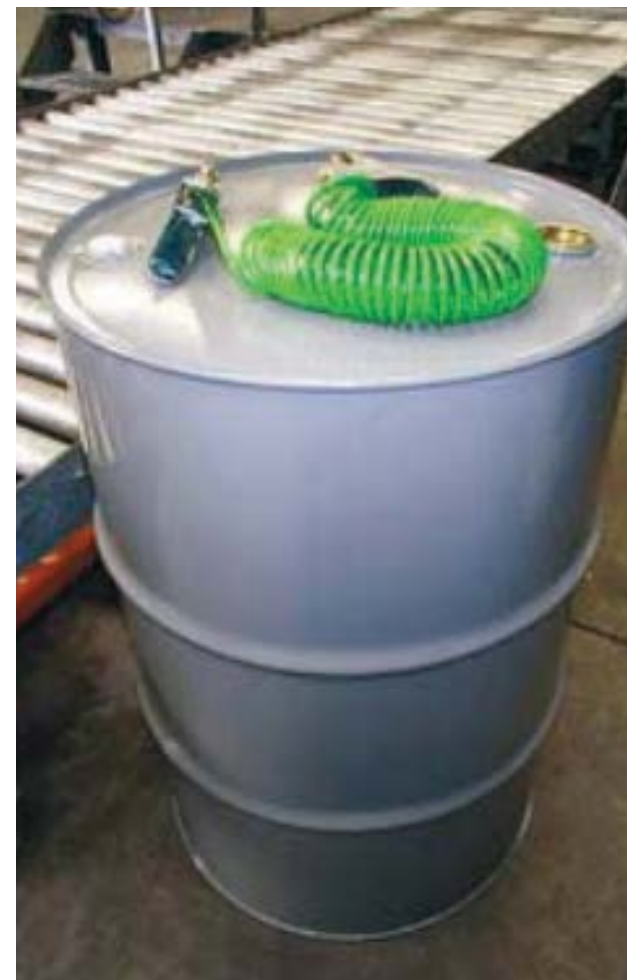
Figure 5. Typical mobile earthing for drums
