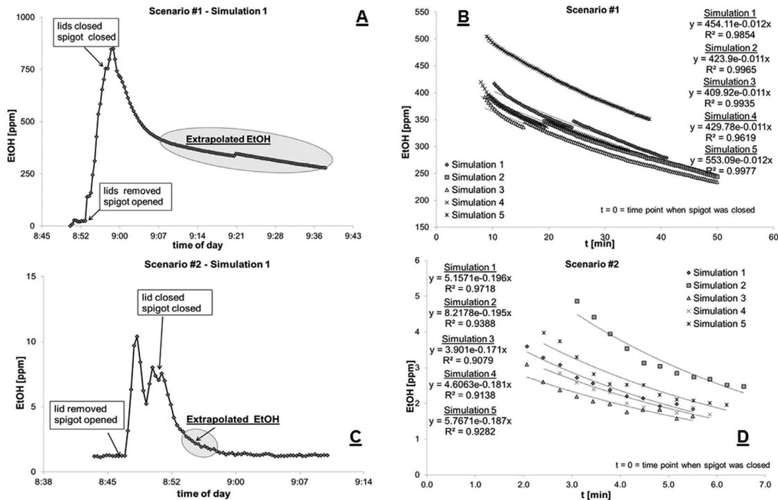
**Figure 2.** Examples of recorded course of airborne ethanol concentration for exposure scenario #1 (A) and #2 (C) as well as the respective graphs for the calculation of EEC (B: exposure scenario #1 and D: exposure scenario #2).
