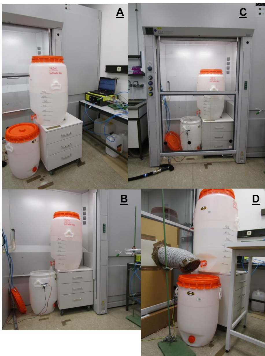
Fig. A 1: Gravity transfer: Experimental set-up for A : Scenario #1, B : Scenario #2, C : Scenario #3 and D : Scenario #4.
