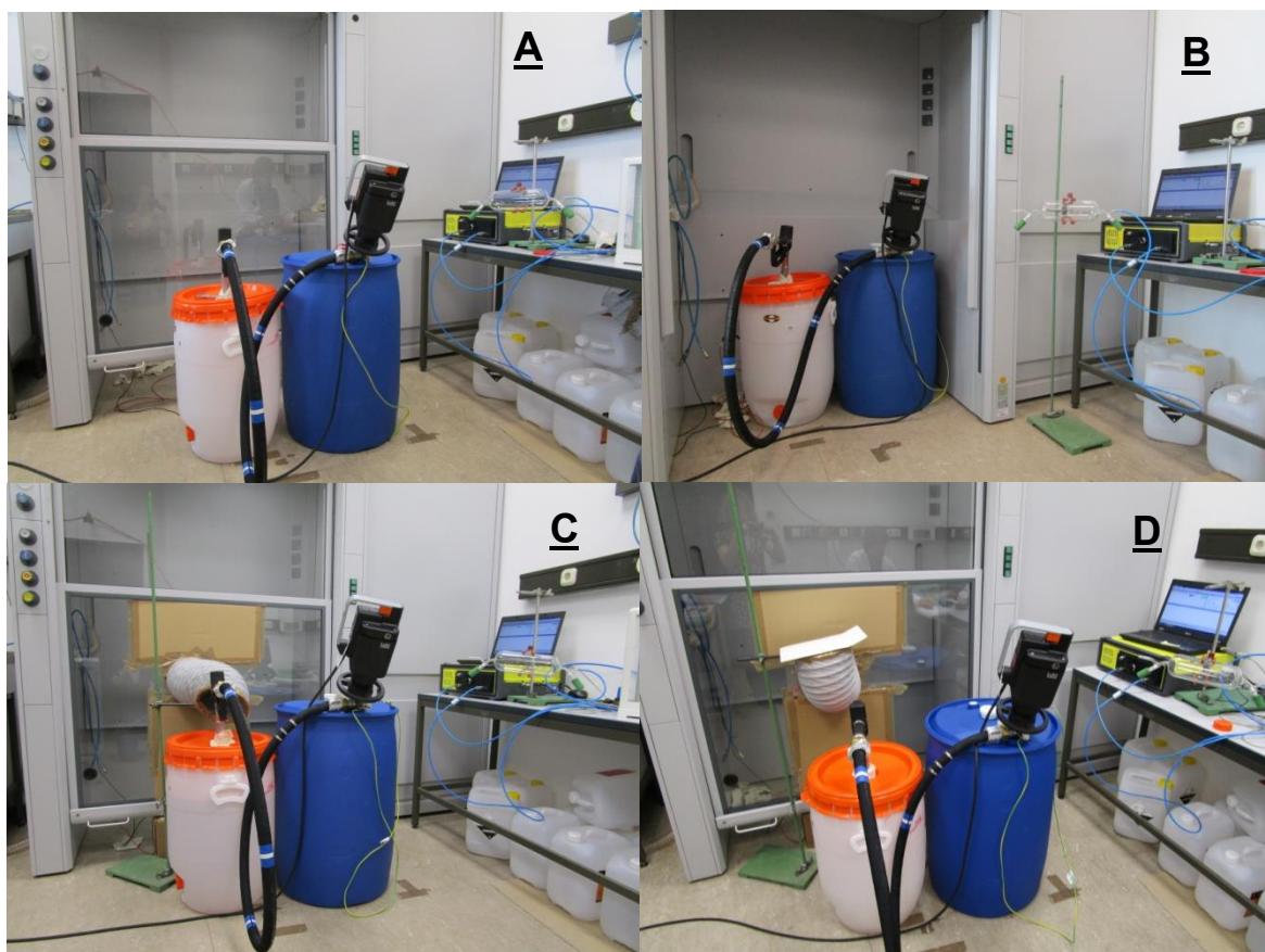
Fig. A 2: Drum pump transfer: Experimental set-up for A : Scenario #5, B : Scenario #6, C : Scenario # 7 and D : Scenario #7a.
