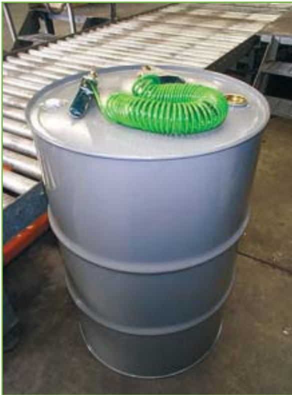
Figure 2. Typical mobile earthing for drums
